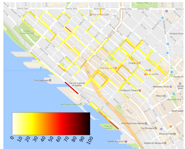
Fig. 10: Locations of average occupancy error between data and simulation across weekdays, March — June 2016
