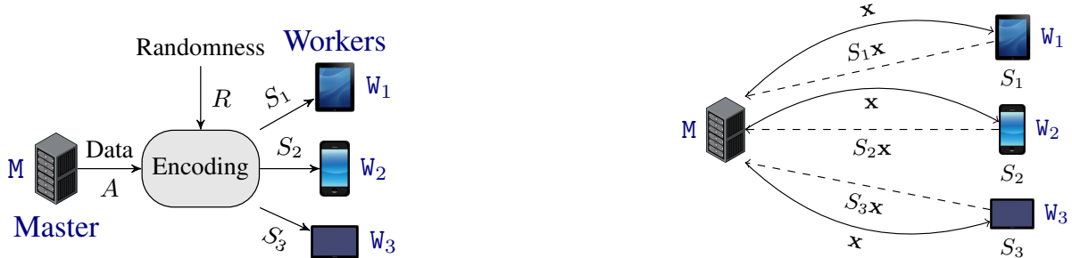
(a) The Master M encodes its data A with a random matrix R into 3 secret shares S_1 , S_2 , S_3 . Any two shares can decode A . For example, S_1 = R , S_2 = A + R , and S_3 = A + 2R . M sends the share S_i to worker W_i . The randomness R is used to ensure privacy.
