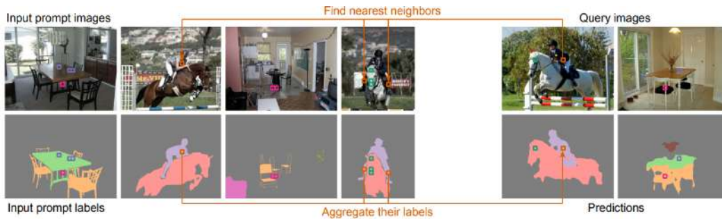
Figure 4.18: Hummingbird (Balažević et al., 2023) is proposed for in-context visual scene understanding through nearest-neighbor retrieval. Image credit: Balažević et al. (2023).
