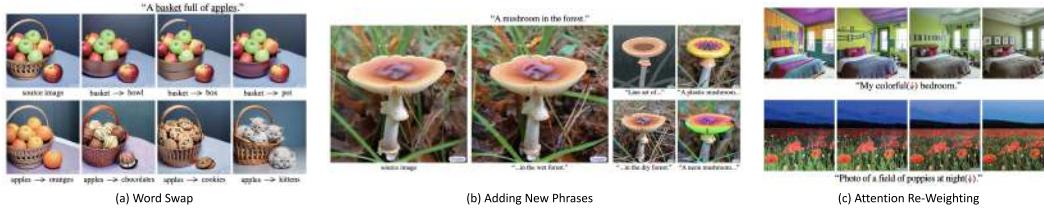
Figure 3.7: Three types of editing (word swap, adding new phrases, attention re-weighting) on synthetically generated images, enabled by attention map manipulation. Image credit: Hertz et al. (2022).
