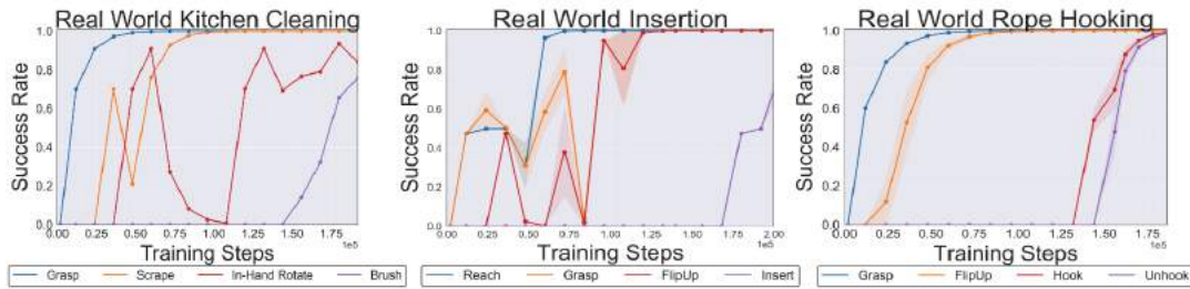
Fig. 6: Success rates of different milestones across our real world dexterous manipulation tasks. Our method is able to perform all the kitchen milestones with around 80% success rate (left), successfully perform pipe insertion (middle, red curve) with around 80% success, and nearly perfectly hook and unhook the rope (right, red/purple curve). Overall, success on other milestones improves earlier in training (blue, orange curves), equipping the robot with skills to autonomously retry the task.
