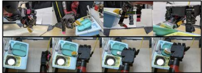
Fig. 12: Sample images for successful Grasp, Scrape, Rotate, Brush task, (each column respectively)
