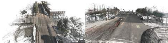
Figure 9. Sample scene reconstruction given lidar points and camera images. We project the lidar points in an image plane with colors assigned based on the pixel color from camera data.
