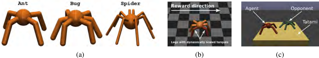
Fig. 2: (a) The three types of agents used in experiments. The robots differ in the anatomy: the number of legs, their positions, and constraints on the thigh and knee joints. (b) The nonstationary locomotion environment. The torques applied to red-colored legs are scaled by a dynamically changing factor. (c) RoboSumo environment.
