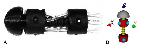
Fig. 2 A: Prototype of the hydraulically driven robot with a drill bit at the front. B: Model of the robot based on geometric primitives and its local coordinate frame.
