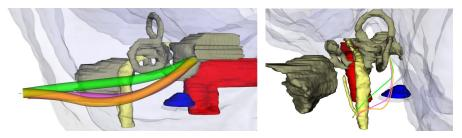
**Fig. 7** RL-Access planned by a standard RRT (pink tube) with safety distance 1.0 mm and by a  $\kappa$ -RRT-Connect (green, orange) with safety distances 1.0 mm and 1.5 mm, respectively.
