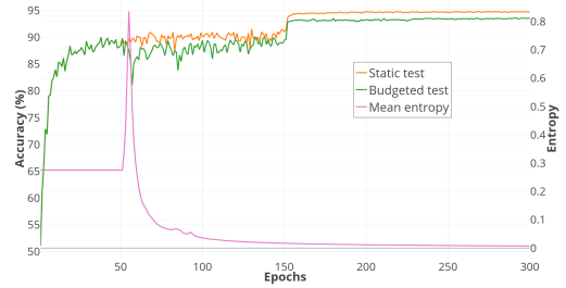
Figure 4: The figure illustrates the evolution of the loss function during learning iterations for CNF and B-CNF, and also the entropy of \Gamma . the period between iteration 0 and 50 is the burn-in phase, at iteration 150, the learning rate has been decreased to increase the convergence speed.
