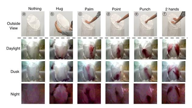
Fig. 9. The six interaction gestures toward an inflatable bladder that were evaluated in our experiments. The top row captured interaction gestures from an external view, whereas the bottom three rows are the image samples from training dataset, captured by an internal camera under three lighting conditions. Images are presented after preprocessing.
