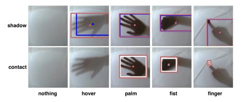
Fig. 13. Results of tracking shadow (1st row) and contact (2nd row) positions on five image frames, each for one gesture. The tracking results are represented using bounding boxes in different color (blue for shadow, and white for contact). The ground truth bounding boxes are constructed manually for each frame (in red color).
