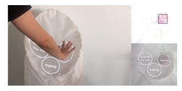
Fig. 17. A robot's skin can be augmented into an interactive touch screen by integrating ShadowSense with a projector. Users can instruct robot by pressing the virtual buttons.
