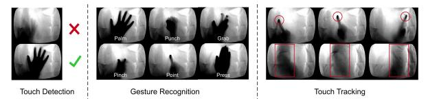
Fig. 3. ShadowSense can (a) detect touch activities, (b) classify touch gestures, and (c) track touch positions.
